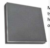
Manufactured (Photonis) as glass plates, typically 4x4 cm, 1mm thick,
