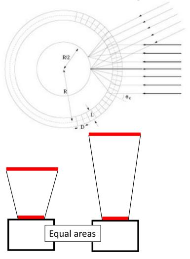
A consequence of the geometry is that the detector geometrical area is ¼ the optic geometrical area.
