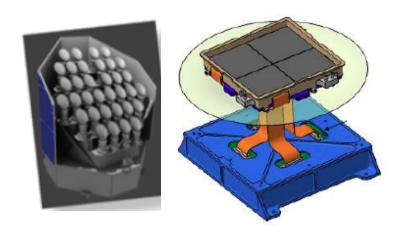
SXI CCDs optimised for X-ray detection e.g. no AR coating, 40 µm depletion depth
